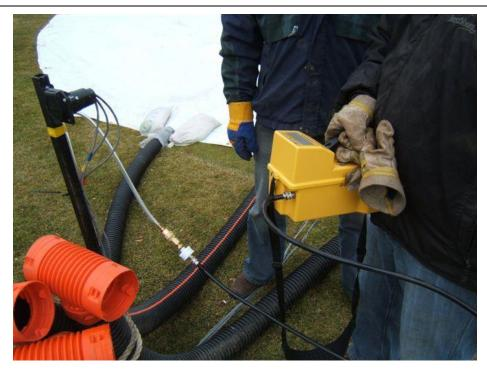
Picture of meter that collected and analyzed oxygen and carbon dioxide.
